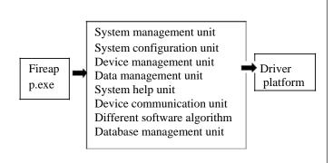
8. The measurement data received by the computer system from sensor node also periodically saved in the database server in the building. Fig: Fire prevention system software design
